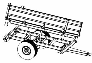
It is possible to tip in rear as well as sideways. The FIELDKING 3 WAY TIPPING TRAILER is therefore provided with hinges at every corner point. Locking pins have been provided for these hinges. Decide the location of the pins according to the side on which tipping will take place. There are three possibilities:
