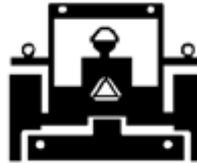
The SMV (Slow-Moving Vehicle) emblem is universal symbol used to alert drivers of the presence of equipment traveling on roadways at a slow speed. SMV signs are a triangular bright orange with reflective red trim for both easy day and night visibility. Make sure the SMV sign is clean and visible from the rear of the unit before transporting the tractor and implement on a public roadway. Replace the SMV emblem if faded, damaged, or no longer reflective.
