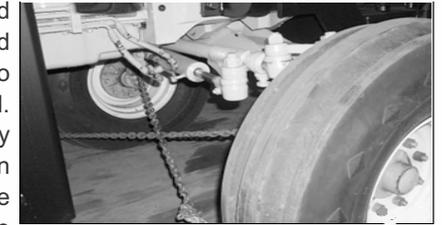
Arrange the chains so that when tightened, the chains are pulling downward and against themselves. Carefully tighten the securing chains or other fasteners using boomers or binders to apply maximum tension. Use extreme care when attaching and removing the securing devices as the extreme tension involved when released has the potential to inflict serious injury.
