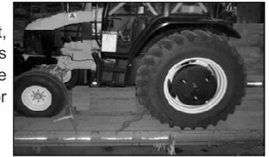
Use adequately sized and rated trailers and equipment to transport the tractor and implement. Consult an authorized dealer to determine the proper equipment required. Using adequately sized chains, heavy duty straps, cables and/or binders, securely tie down both the front and rear of the tractor utilizing the proper tie down locations as specified by the tractor manufacturer.
